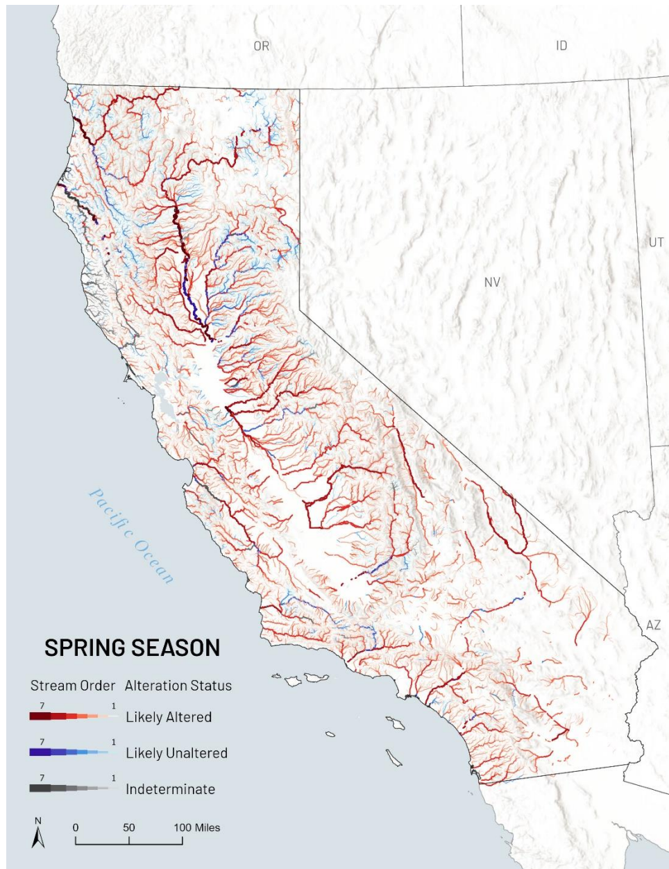
Figures S2: Map of spring recession flow alteration for all COMIDs in California based on the functional flow metrics calculated from the Actual flows model daily streamflow time series. Red indicates likely altered where at least one metric within the flow component (timing, duration, magnitude, rate of change) was identified as altered. If none were likely altered, but at least one metric within the flow component was identified as indeterminate, the color grey indicates that alteration status is indeterminate. All other COMIDs were classified as likely unaltered. Width of the line indicates stream order.
